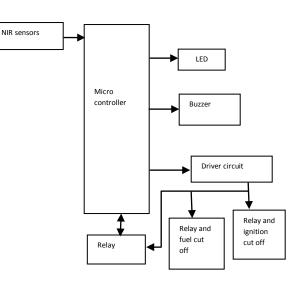
The same can be implemented in the two wheelers by just placing the NIR sensors on the accelerator of the vehicle and it follows the same circuit
